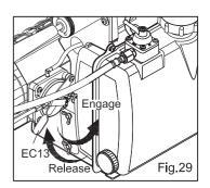
Start the engine once more. Engage the lever and open solution tap (120), fog should be seen emitted. (Fig. 30)
