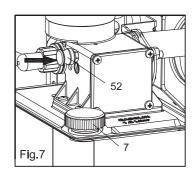
7) Tighten the drainage cap before filling solution tank (1). Always use solution funnel (143) with strainer. (Fig. 8)
